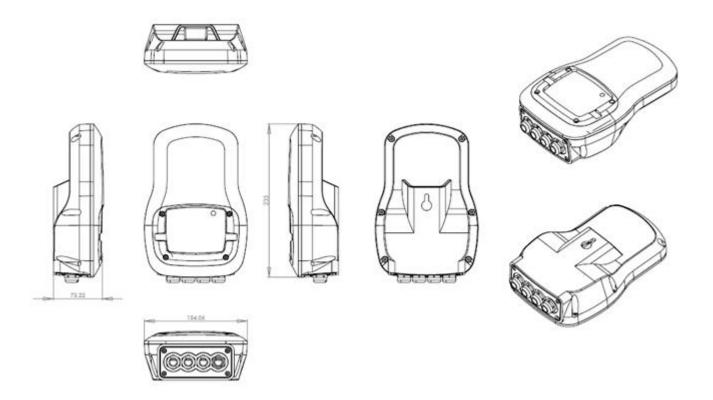
The connections to the **EnCompay** are via cable entry holes in the bottom of the case, where cables pass through glands and terminate into the spring loaded plug-in terminals mounted on the edge of the printed circuit board. The case has a detachable plate that is screwed, complete with seal. This plate can be replaced with a blank or with 4 or 8 holes (See below).
